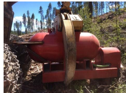
Figure 8: Wildfire Prevention – (Mobile Grapple Skidder Watertank/ Pump Unit)
